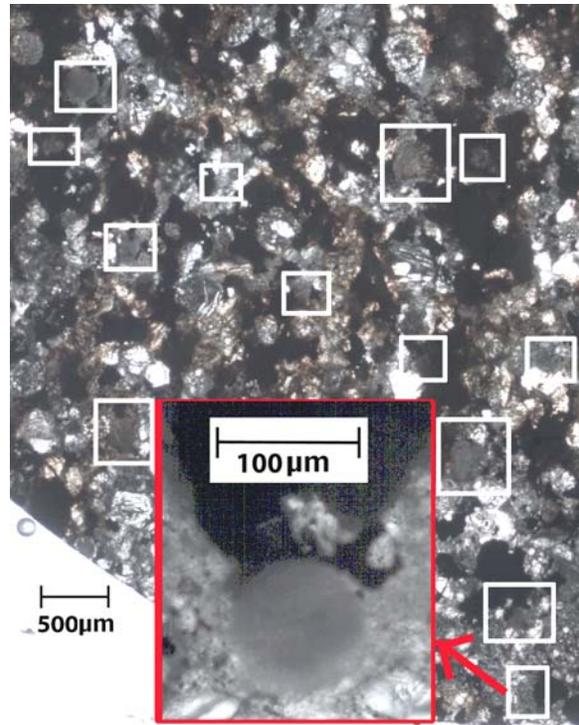
Fig. 5. Transmitted light image of a region along the bottom left of Fig. 1. White boxes surround some of the cryptocrystalline chondrules in this region.
