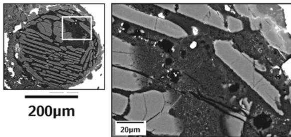
Fig. 4. BSE image of a mixture of turbid and clear glass in the mesostasis of a barred olivine chondrule. The white areas are opaques, light gray is olivine, dark gray is glass, medium gray (upper right) is pyroxene.
