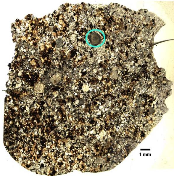
Fig 1. Petrographic thin section (BC1) of Buzzard Coulee. A large cryptocrystalline chondrule is circled.
